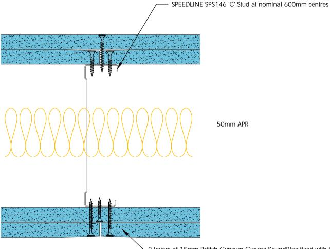
2 layers of 15mm British Gypsum Gyproc SoundBloc fixed with SPEEDLINE Drywall Screws at 300mm centres (200mm centres at external angles). Ref to table for fixing length.
